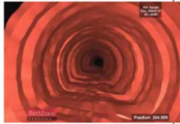
Figure 1: Sonar inspection image Source: Redstone 2007, http://redstone.com/
